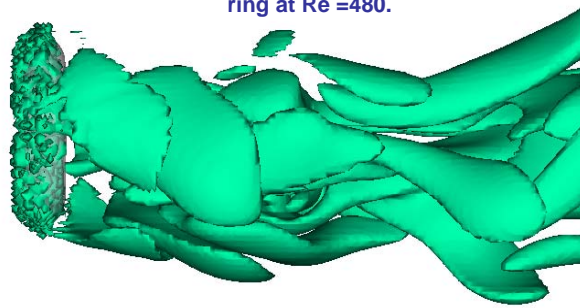
Three-dimensional (3D) vortex shedding in flow past a toroidal ring at Re=480 .
