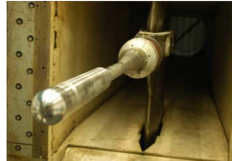
Top picture: Hemispherical head cylinder in a supersonic wind tunnel.
